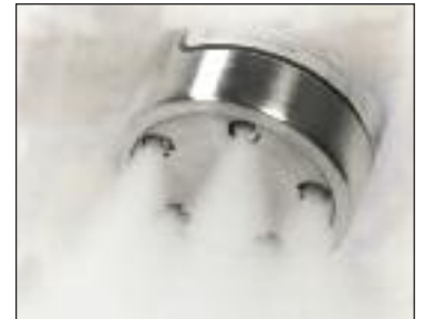
Aerosol generator discharge
