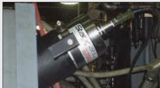
Stat-X automatic generators protecting CNC machine with an externally mounted aerosol unit.
