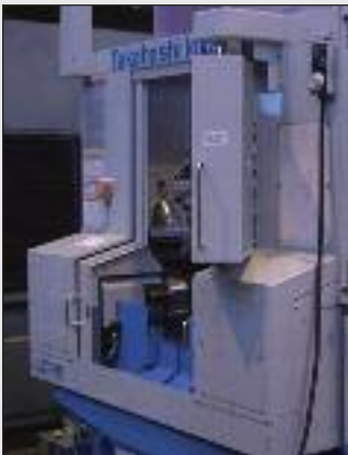
Stat-X fixed system protecting CNC machines with internally mounted aerosol unit.
