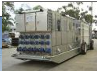
Mobile mining substation and switch gear
