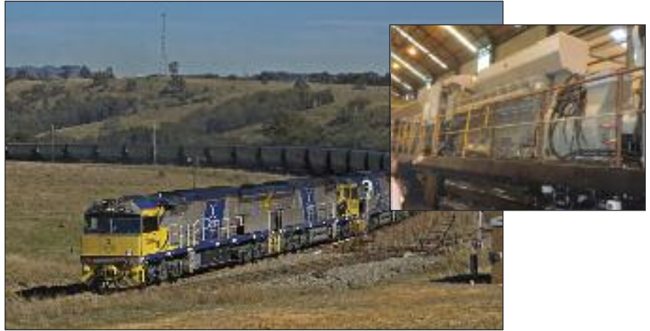
Stat-X® Fire Suppression System protects the engine and alternator cabs and the oil filter compartment.
